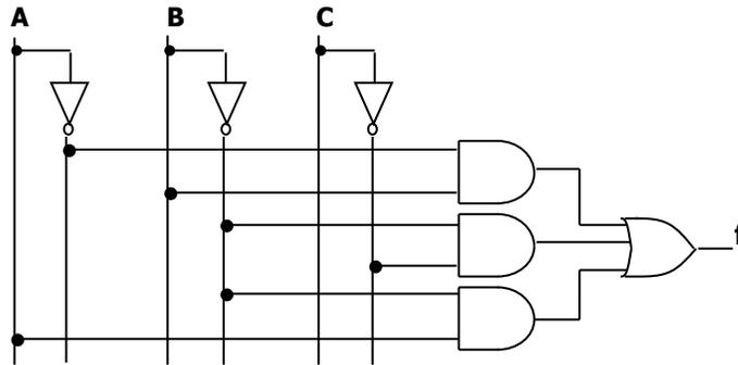
✓  $F(A, B, C) = \prod(M_0, M_3, M_5, M_7) = \sum(m_1, m_2, m_4, m_6) = \bar{A}\bar{B}C + \bar{A}B\bar{C} + A\bar{B}\bar{C} + AB\bar{C} = \bar{A}\bar{B}C + \bar{C}(\bar{A}B + A\bar{B} + AB)$
