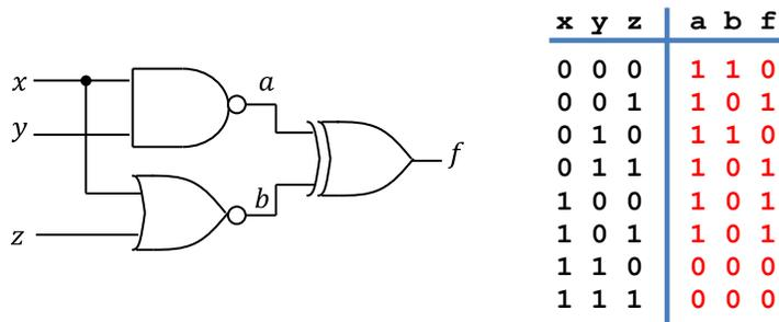
$$f = \bar{a}\bar{b} = a \oplus b = (xy) \oplus (x+z) = (\bar{x}\bar{y})(x+z) + xy(\bar{x}+\bar{z}) = (\bar{x}+\bar{y})(x+z) + xy(\bar{x}\bar{z}) = (x+z)(\bar{x}+\bar{y}) = \bar{x}z + x\bar{y}$$
