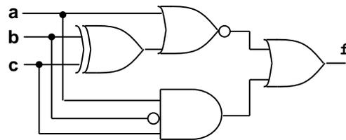
$$f = \bar{a}\bar{b}c + \bar{a}bc + a\bar{b}c = \bar{a}(b \oplus c) + a\bar{b}c = \bar{a} + (b \oplus c) + a\bar{b}c$$
